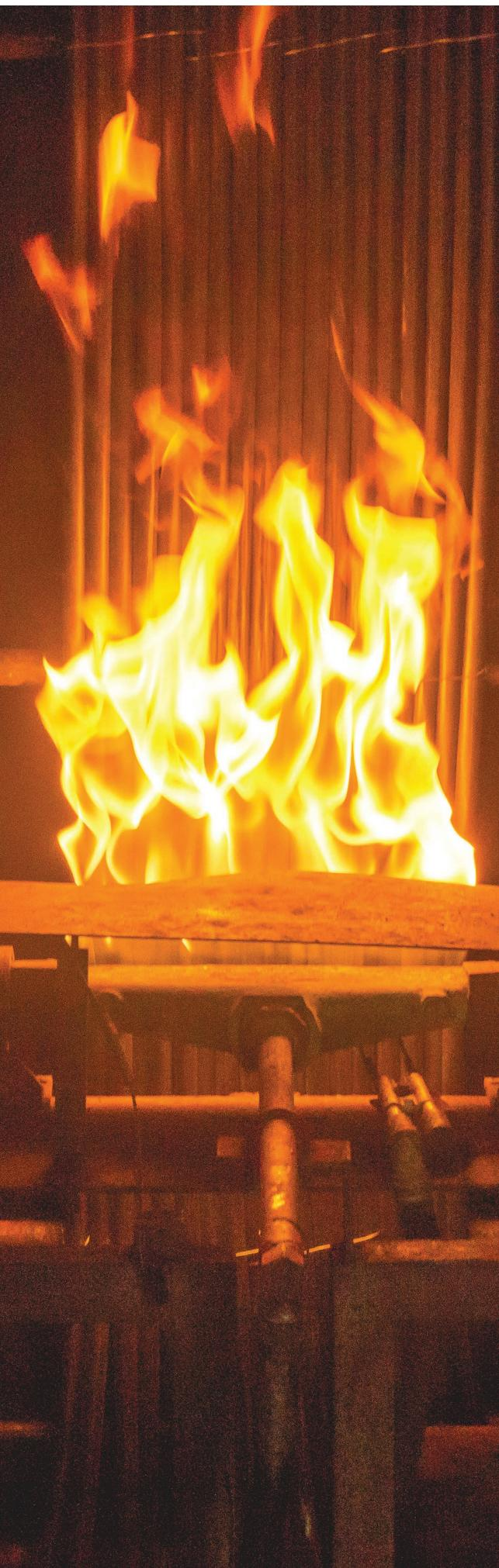
**IEC 60332-1-2 : TESTS ON ELECTRIC AND OPTICAL FIBRE CABLE UNDER FIRE CONDITIONS - PART 1-2: TEST FOR VERTICAL FLAME PROPAGATION FOR A SINGLE INSULATED WIRE OR CABLE - PROCEDURE FOR 1 KW PRE-MIXED FLAME**
