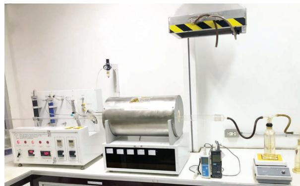
**IEC 61034-2 : MEASUREMENT OF SMOKE DENSITY OF CABLES BURNING UNDER DEFINED CONDITIONS - PART 2: TEST PROCEDURE AND REQUIREMENTS**
